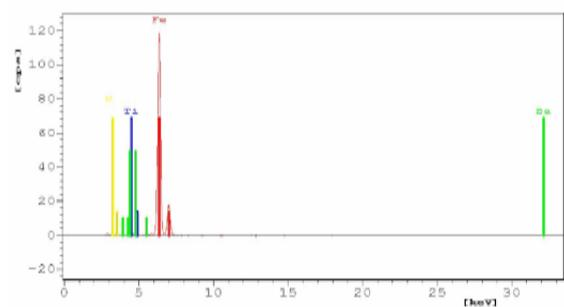
Fig. 5. X-ray fluoresce (XRF) spectroscopy of anthill clay
