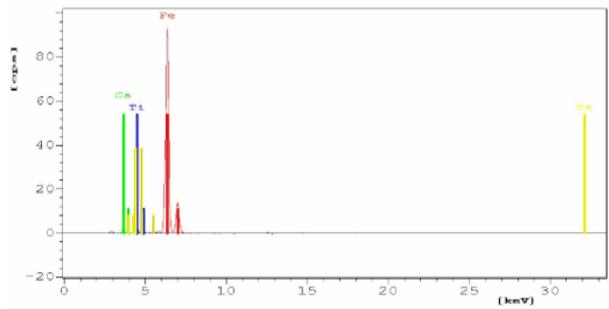
Fig. 6. X-ray fluoresce (XRF) spectroscopy of brick clay
