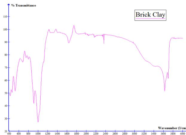
**Fig. 9.** FT-IR spectroscopy (transmittance) of brick clay
