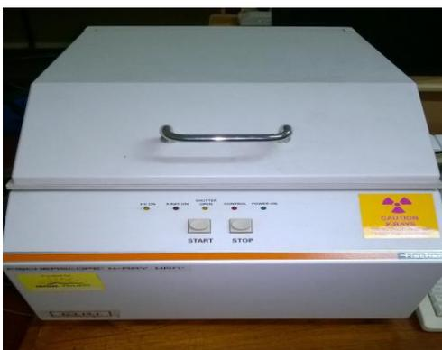
Fig. 3. X-ray fluorescence (XRF) spectrometer
