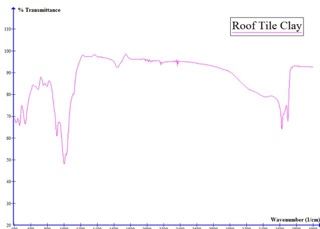
Fig. 10. FT-IR spectroscopy (transmittance) of roof tile clay
