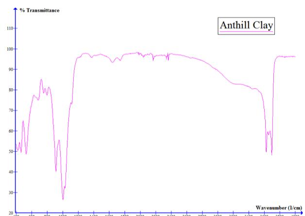
Fig. 8. FT-IR spectroscopy (transmittance) of anthill clay
