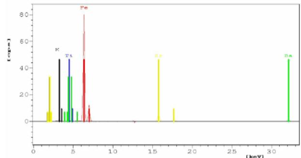
Fig. 7. X-ray fluoresce (XRF) spectroscopy of roof tile clay
