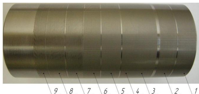
Fig. 1. Surfaces of VT22 after ultrasonic burnishing on different conditions.
