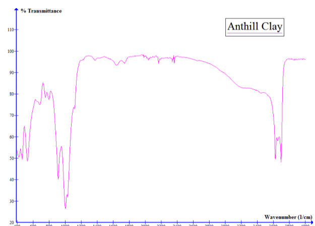
Fig. 8. FT-IR spectroscopy (transmittance) of anthill clay
