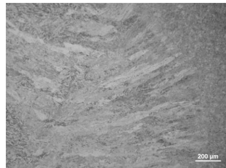
Fig. 5. Structure of clad layers sample A
