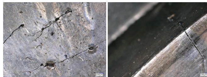
Fig. 2. Cracks on the mold surface
