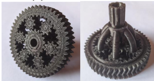
Fig. Model of the planetary gear train with the herringbone gears, manufactured with additive technology. (The specimens and their photographs have been rendered by V. Dubrovskii).
