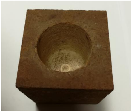
Fig. 2 Crucible constructed from magnesia refractories
