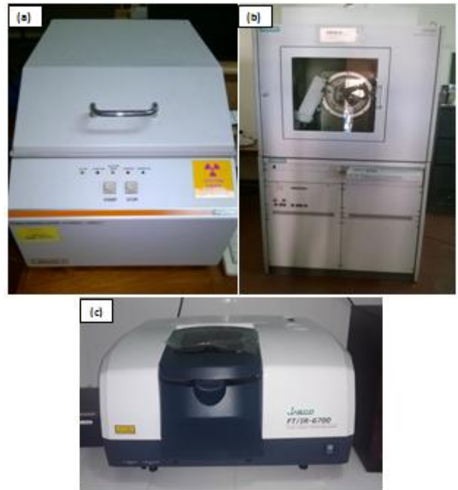
Fig.7. (a) X-ray fluorescence (XRF) spectrometer, (b) X-ray diffraction (XRD) spectrometer and (c) Fourier transforms infrared (FT-IR) spectrometer
