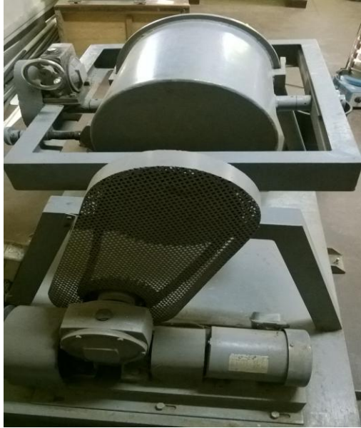
Fig.5. Ball mill (comminution machine)
