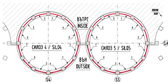
**Fig. 11** Scheme of sequence of the repairation works
