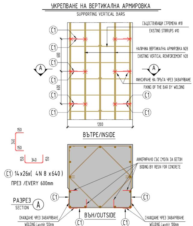
Fig. 5 Existing bars fixing
