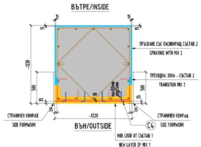
Fig. 7 Repaired section
