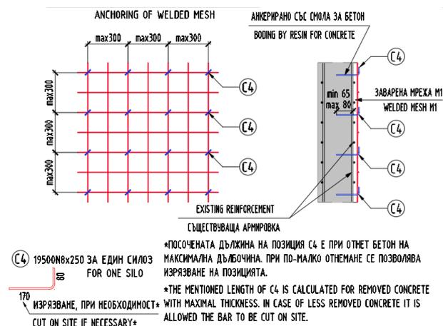
**Fig. 10** Anchoring rods for reinforcing mesh
