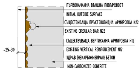
**Fig. 13** Removing concrete cover to reach healthy concrete
