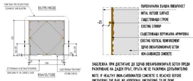
Fig. 6 Second stage of preparing – removal of carbonated concrete
