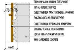
**Fig. 9** Second phase of carbonated concrete removing in the cylindrical body
