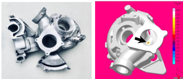
Fig. 1 Aluminium Turbocharger Housing (a)-general appearance and transverse incisions illustrating complexity; (b)-View of the casting with the place and size of the defect
