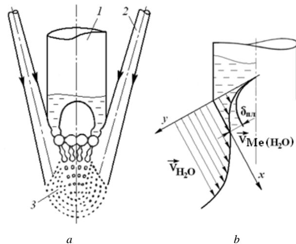
**Fig. 1.** Model scheme for atomization of liquid metal jet (a) and velocity distribution in a water-metal system (b): 1 - stream of metal; 2 - annular flow of water; 3 - cooling zone of metal droplets;  $V_{H_2O}$  - water flow speed;  $V_{Me(H_2O)}$  - speed of metal stream;  $\delta_{pl}$  - metal film thickness
