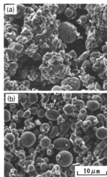
Fig. 5. SEM micrographs of Cu-10% Sn alloy powders produced by high-pressure water atomization using traditional technology (a) and ring nozzle with rotating jet (b) [7]
