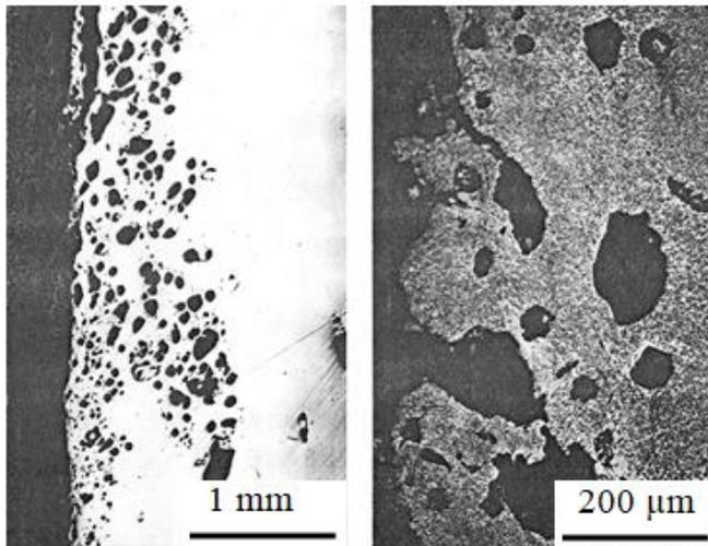
Fig. 3. Macro (a) and microstructure (b) of the subsurface layer of crystallized section of melt jet flame for water atomization of P6M5 high speed steel
