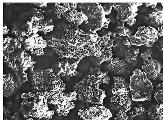
**Fig. 2.** Coral-shaped particles of 50Mn-12Si-17Ni-9Fe powder
