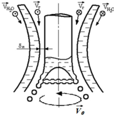
**Fig. 6.** Flow separation scheme for atomization using a vortex type nozzle:  $V_{H_2O}$  - velocity of the water conical stream;  $V_r$  - velocity of the ejected gas (air);  $\delta_n$  - the gap between the water and the jet of melt;  $V_\theta$  - circular rotation velocity of the air-water stream
