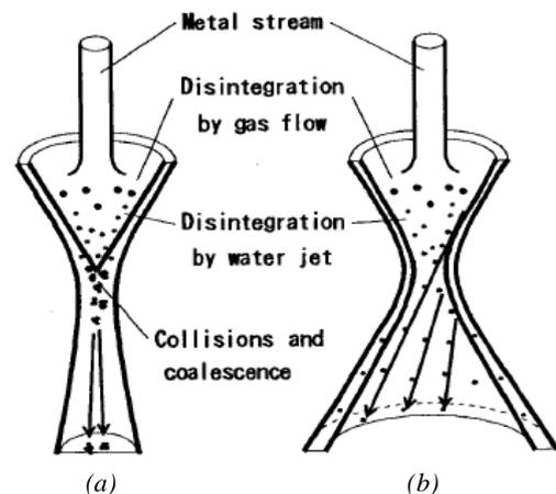
**Fig. 8.** Models of high-pressure water atomization using a direct-flow nozzle (a) and a vortex-type nozzle [7]
