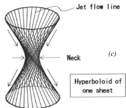
Fig. 4. Schematic cross-section of water jet for water atomization in air-water whirlwing (a) and schematic diagram of air-water stream (b, c) [7]
