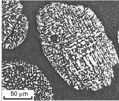
**Fig. 8.** The microstructure of ferromanganese powder produced by water atomization using a vortex type nozzle
