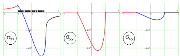
Fig.8 Strands on the surface of the active body in contact with the case C_1 = 3500 \frac{N}{mm^2}, \mu = 0.2
