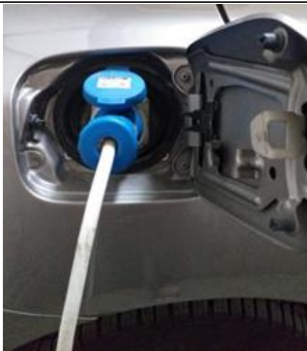
Fig. 6 Charging the electric car with the on-board charger.
