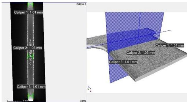
Fig. 11 Measurement of specimen thickness after sharpening.
