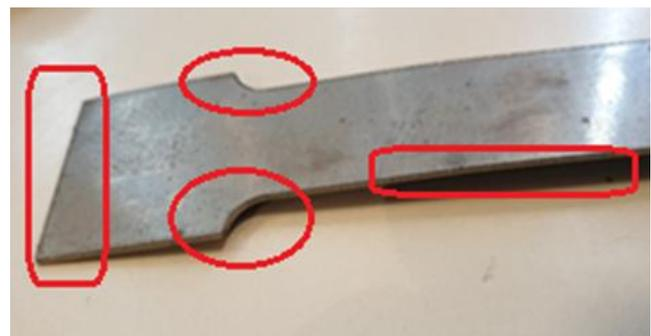
Fig. 2 Test specimen with edges (before punch sharpening).
