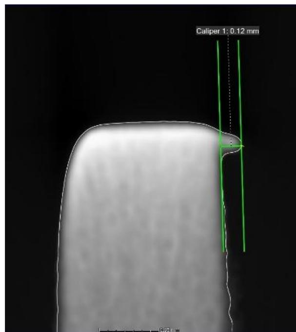
Fig. 4 Defect of the test specimen after punching.
