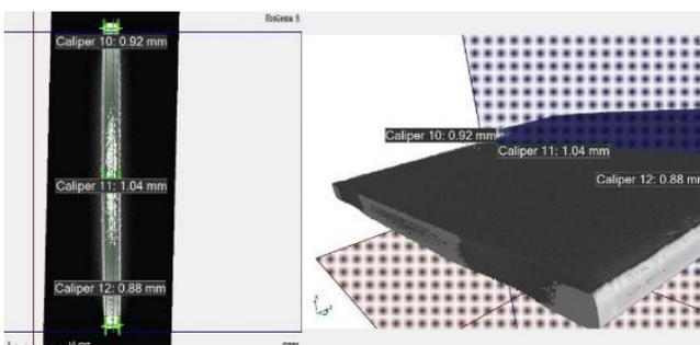
Fig. 9 Measurement of specimen thickness before sharpening.
