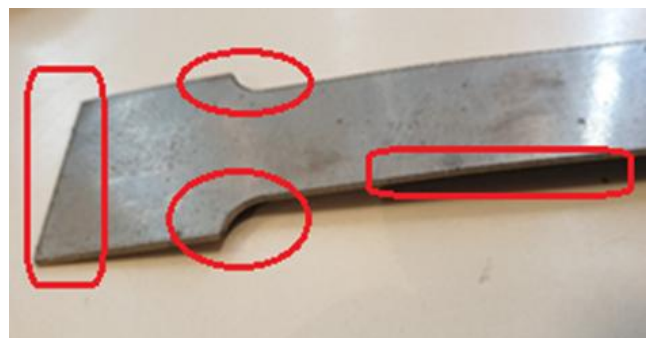
Fig. 2 Test specimen with edges (before punch sharpening).
