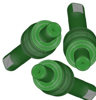
Fig. 2 Model of rolls of radial-shear rolling mill
