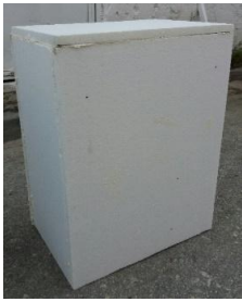
Fig. 4. Sample covered by EPS
