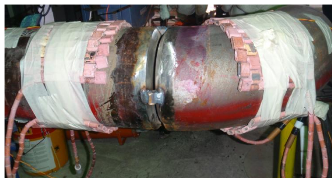
Figure 2. Preheating procedure of a seamless pipe p91.
