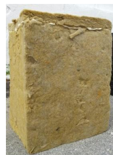
Fig. 3. Sample covered by rock wool
