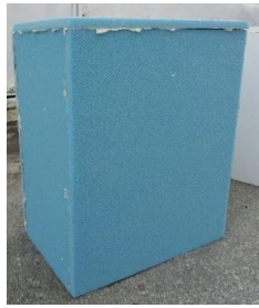
Fig. 5. Sample covered by XPS
