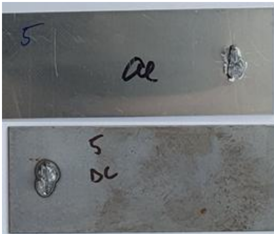
Fig. 4 Appearance of the contact surfaces with the connecting element after the tensile test
