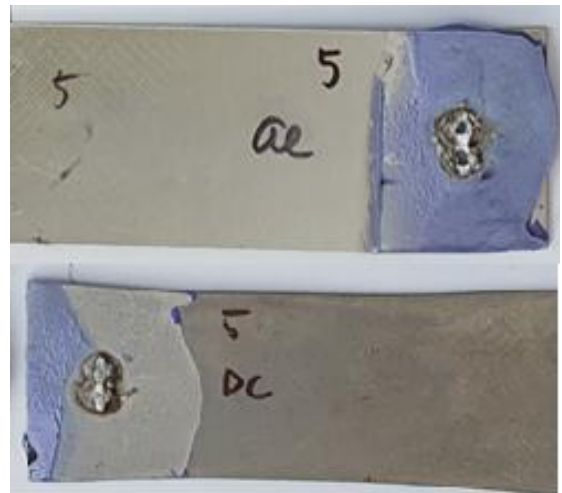
Fig. 8 Appearance of contact surfaces with connecting element and with additional adhesive layer TEROSON EP 5090
