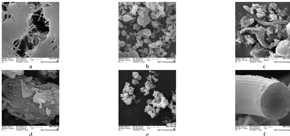
Fig. 2. Typical morphology of particles of PTFE (a), UPTFE (b), carbon nanotubes (c), tripoli (d), metal oxides (e), carbon fiber (f) in the as-received condition
