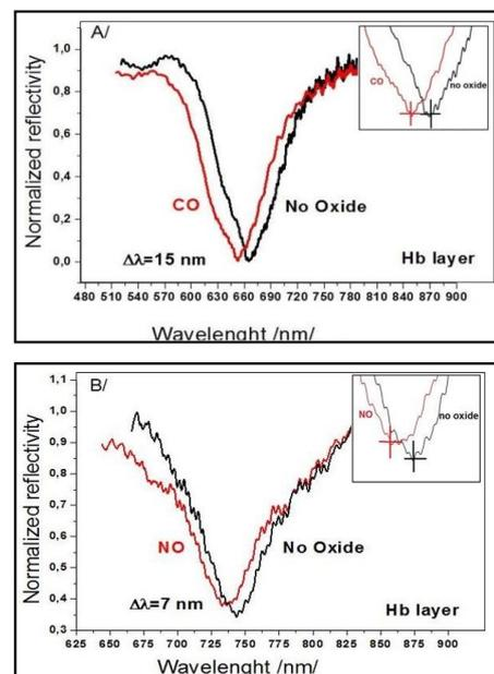
Figure 3. SPR detection of the binding activity of a Hb layer deposited by MAPLE technique
