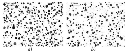
**Fig. 3** Microstructure of ductile iron
