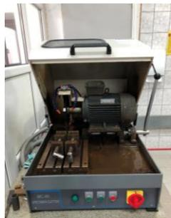
**Fig. 1** Device for cutting specimens.
