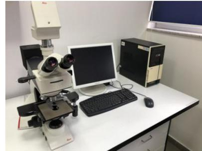
**Fig. 2** Light microscope Leica DM 2500 M.
