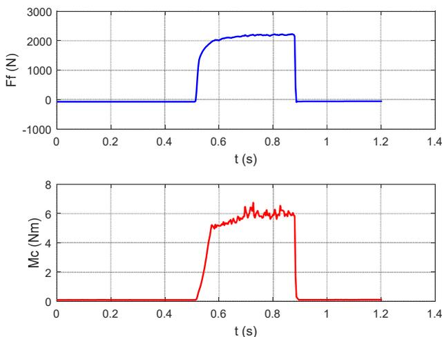
**Fig 6** Cutting forces values at the point of the experimental plan number 7..
