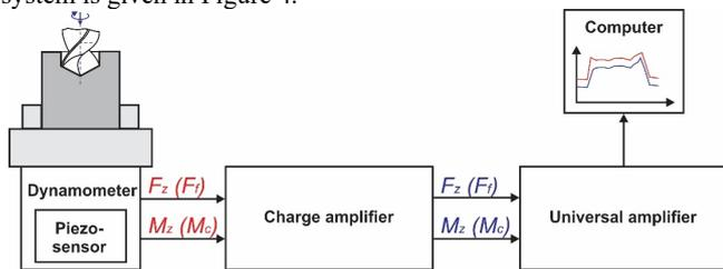
Fig 4 Information measurement system for measuring cutting forces at drilling
