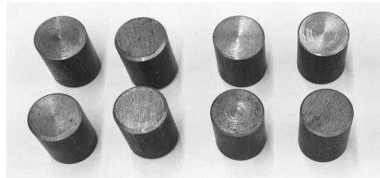
Fig 1 Experimental workpieces made of medium alloyed carbon steel C45
