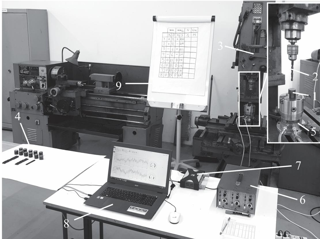
**Fig 5** Research site: 1 – workpiece, 2 – cutting tool (twist drill), 3 – machine (drill press BD-40), 4 – workpieces and tools for experimental points, 5 – sensor (piezo-electric dynamometer), 6 – charge amplifier, 7 – universal amplifier, 8 – a computer with acquisition software, 9 – experiment matrix plan
