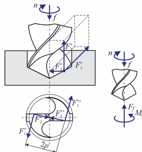
Fig 2 Cutting forces at drilling
