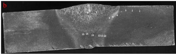
Fig. 5. Location of indentation for Vickers hardness test, GMAW weld joint (a); MCAW weld joint (b)
