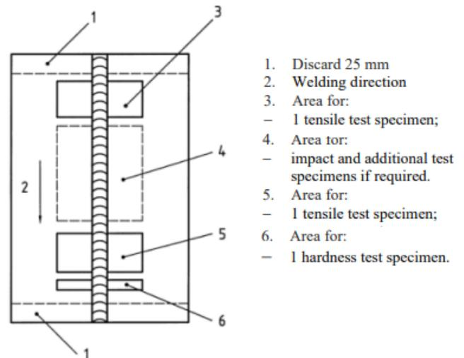
**Fig. 1.** Location of test specimens for a butt joint in plate [5]
