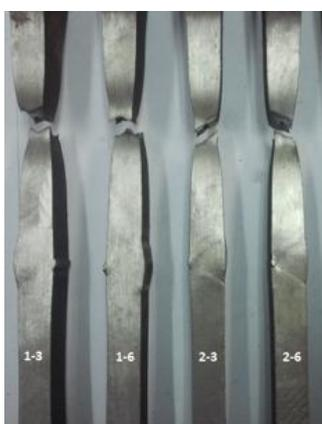
Fig. 2. Tensile test specimens after testing
