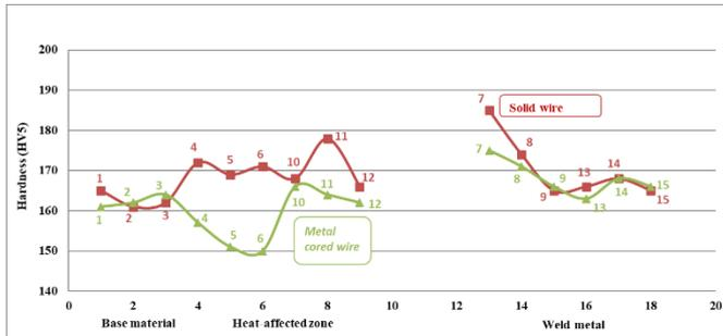
Fig. 6. Measured values of Vickers hardness test HV5
