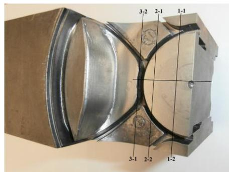
Fig.3 Sampling procedure from the mold part
