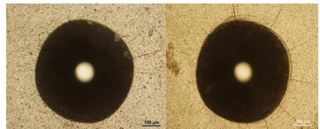
**Fig.7** Indentation impression after Mercedes test; AlN<sup>3</sup> (left), nACr<sup>3</sup> (right)
