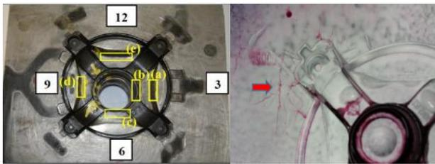
**Fig.4** Worn solid half of the mold insert (left); appearance of cracks of the mould after capillary test by capillary method (right)
