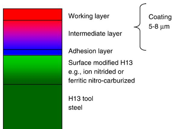
Fig.2 A diagram of an optimized coating architecture for die coatings used in aluminum high pressure die-casting.
