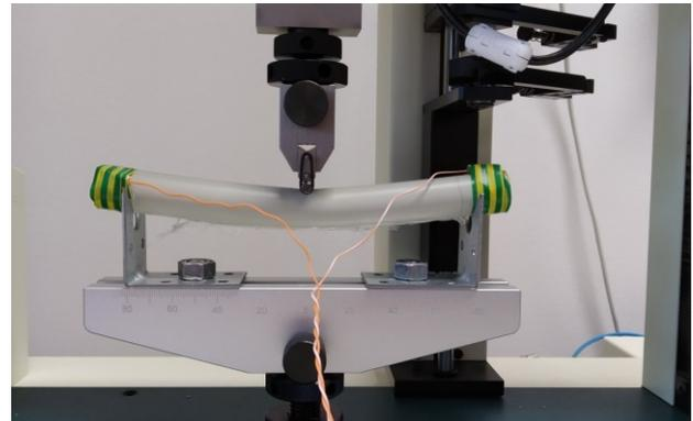
Fig.1. Three-point bend test arrangement
