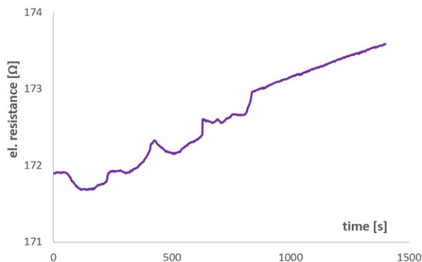
Fig.4. Recording the electrical resistance of the nitinol wire placed on the tube transversely in the wraps during deformation
