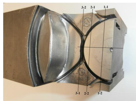
Fig.3 Sampling procedure from the mold part
