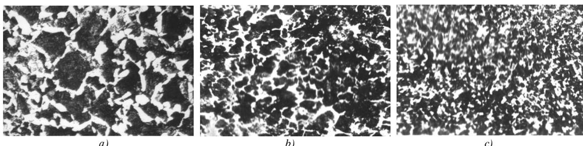
Fig. 2. Microstructure of AISI-5140H steel: a – initial, b – shaped in flat strikers, c – shaped in a new forging tool
