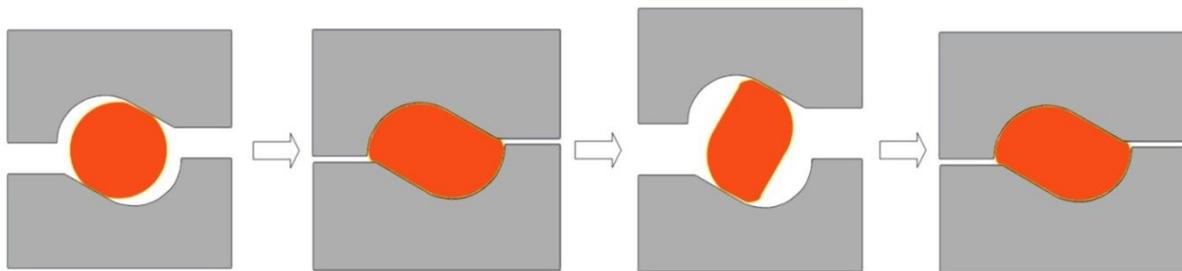
Fig. 1. Forging tool and scheme workpiece deformation
