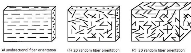
Fig. 2 Example of reinforced fiber orientation [5].
