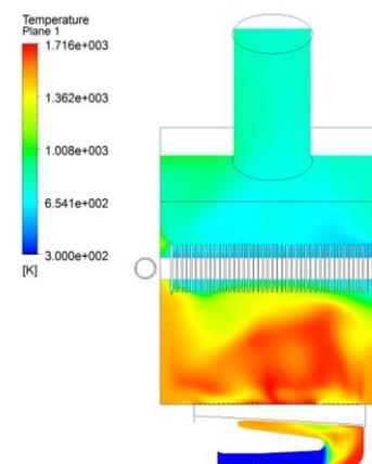
**Fig. 6** Simulation of temperature change in the working process of the original designed combustion system of the innovative commercial dishwasher prototype.
