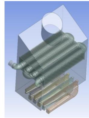
**Fig. 4** Originally designed combustion system of the innovative commercial dishwasher prototype.
