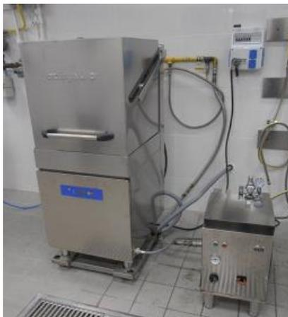
Fig. 8 Front view of the innovative commercial dishwasher prototype.
