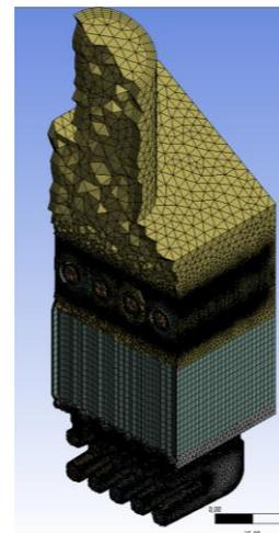
**Fig. 5** The view of the mesh distribution in the original design combustion system design.
