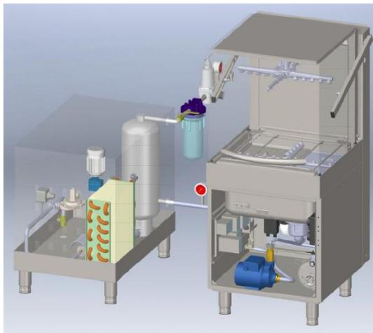
**Fig. 3** The draft drawing of the commercial dishwasher prototype using gas-heated water.
