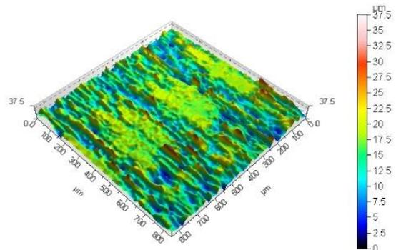
Fig. 8 3D picture of the tribo wear track on sample 03 produced by the Pin-on-Disc test
