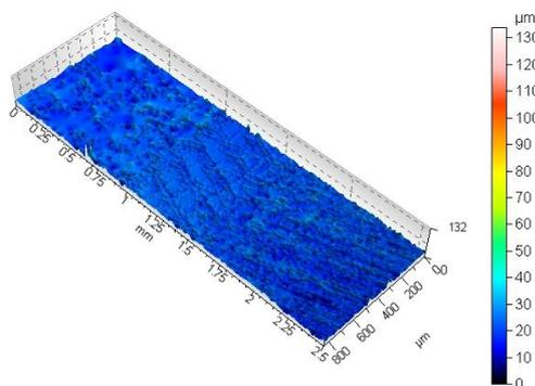
Fig. 6 3D picture of the tribo wear track on sample 01 produced by the Pin-on-Disc test
