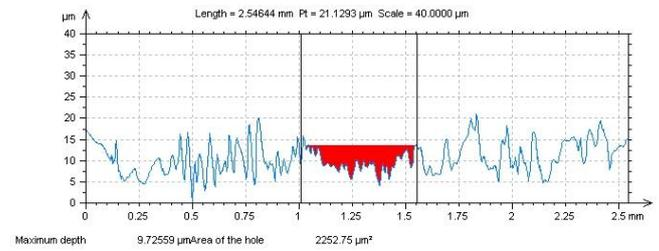
Fig. 7 Scheme of the tribo wear track on sample 03 produced by the Pin-on-Disc test
