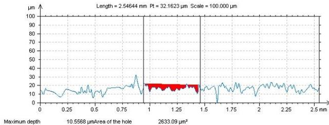
Fig. 5 Scheme of the tribo wear track on sample 01 produced by the Pin-on-Disc test
