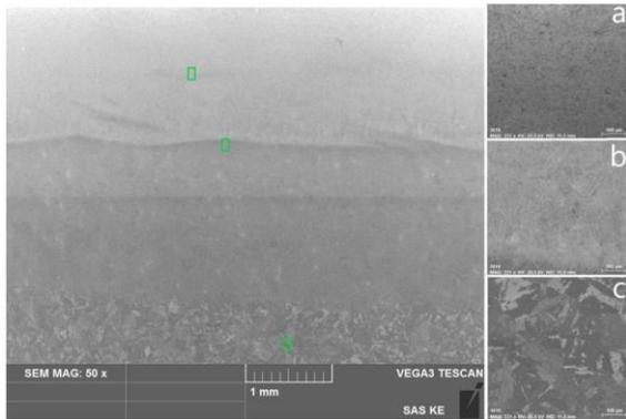
Fig. 4 Weldment 03. Electron microscope image, capturing the interface of a) weld metal, b) heat affected area, c) base material
