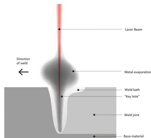
Figure 1. Schematic representation of laser beam welding [13]
