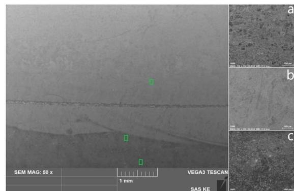
Fig. 3 Weldment 01. Electron microscope image, capturing the interface of a) weld metal, b) heat affected area, c) base material
