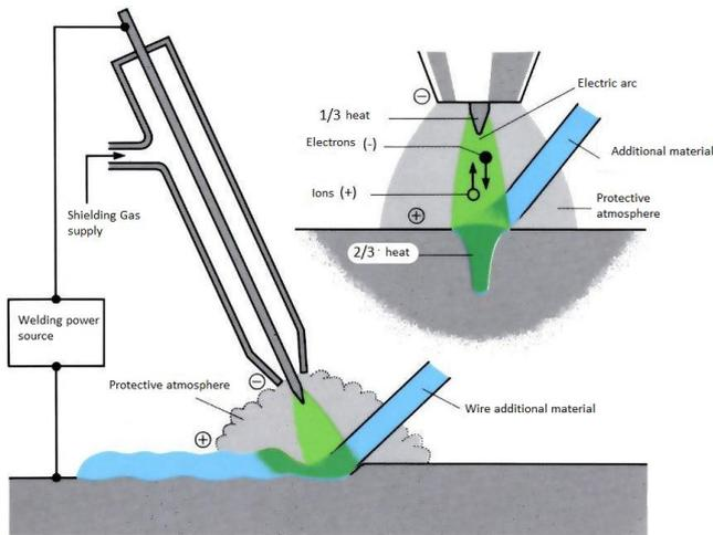
Fig. 2 Schematic representation of the MIG / MAG method [18]
