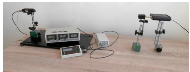
Fig. 2 Device for measuring the number and diameter of fog drops (Fog Detector 6).
