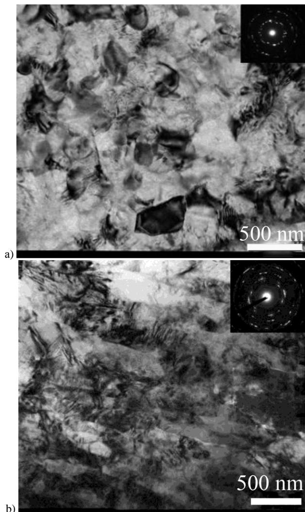
**Fig. 1.** Titanium structure after radial shear rolling up to a diameter of 15 mm and cooling in water: a - peripheral part of the bar; central part of the bar
