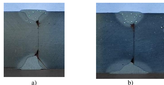
Fig. 4. Imprints of the indenter by the specimens: a) cooled in air, b) cooled in water
