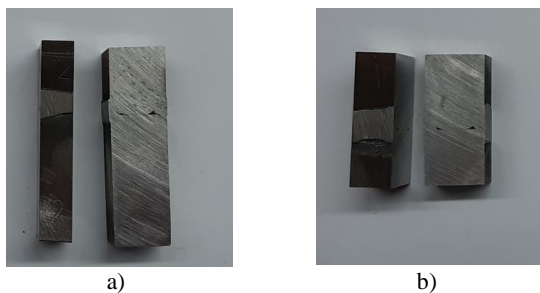
Fig. 3. Cut specimens: a) air-cooled joint, b) water-cooled joint
