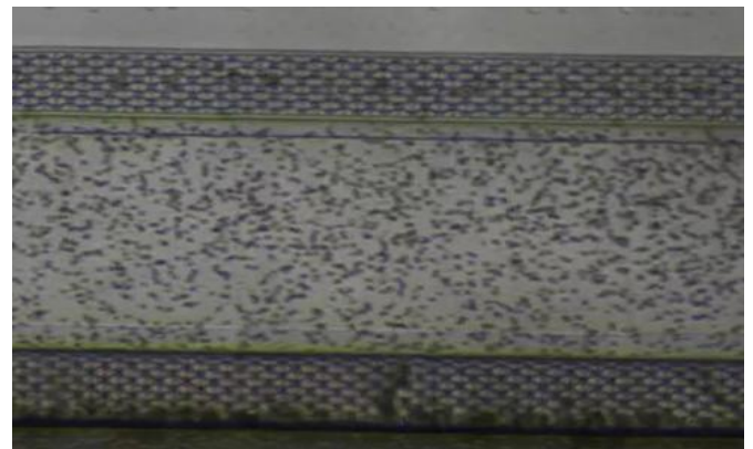
Fig. 7 Image of the developed microchannel filled with a diluted erythrocyte suspension.
