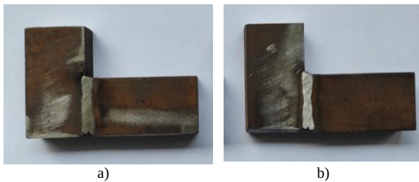
Fig. 2. Specimens: a) cooled in air and b) cooled in water
