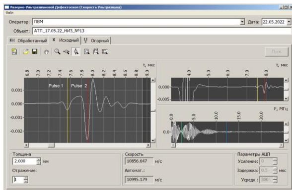
Figure 7. Screenshot of the UDL-2M screen. Measuring the thickness of the diamond layer. The time difference between pulse 1 and pulse 2 allows you to calculate the thickness of the diamond layer. In this case, it is 4 mm.
