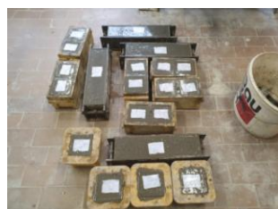
Fig. 5 Concrete test specimens prepared
