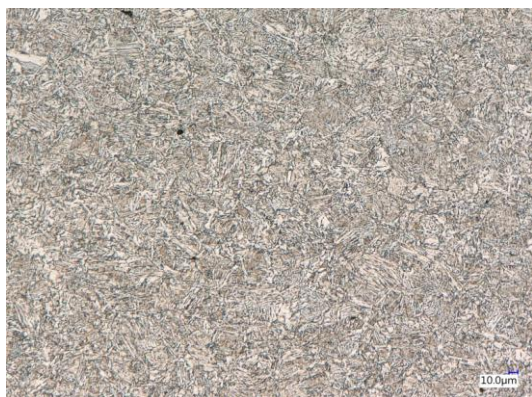
Fig. 24 Microstructure of weld metal from pipe No. 2
