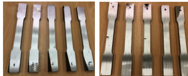
Fig. 5 Samples before tensile test
