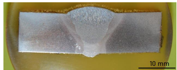
Fig. 21 Macrostructure of the weld of the sample from tube No. 2
