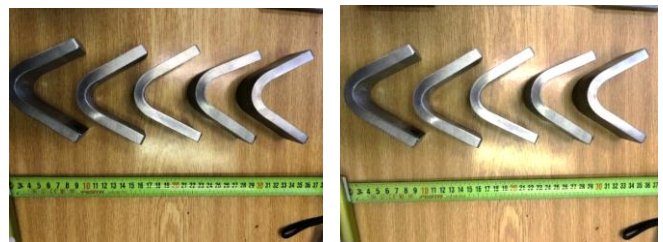
Fig. 14 Test specimens after bend test
