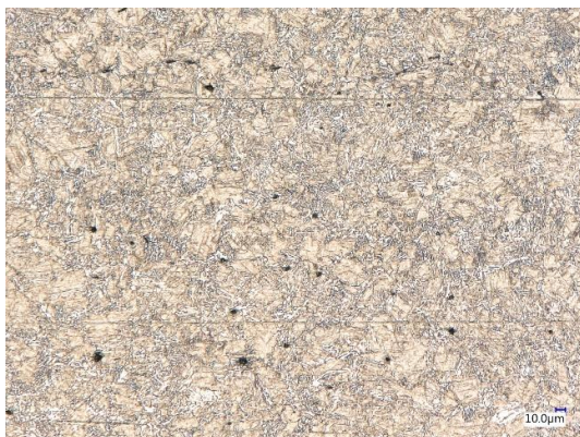
Fig. 23 Microstructure of the HAZ (heat affected zone) of tube No. 2
