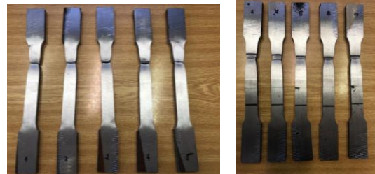
Fig. 13 Samples after tensile test
