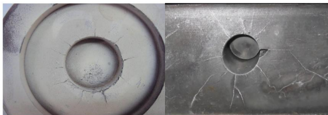
Fig. 1 Initiation and propagation of cracks due to thermal gradient of the mould surface
