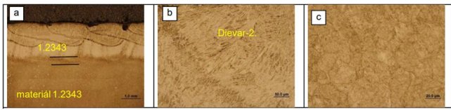
Fig.2 Material 1.2343-Dievar, a) disposition; b) detail of the outline; c) background material
