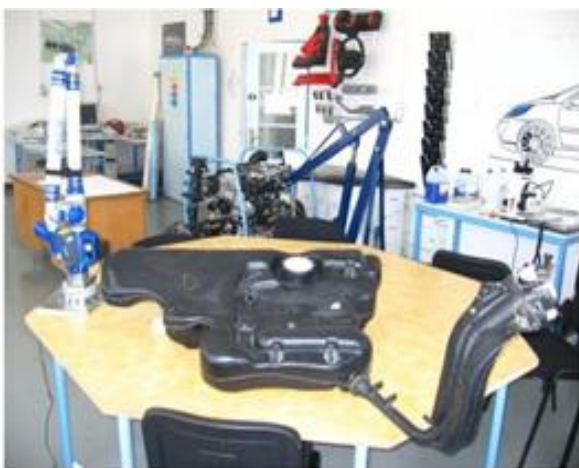
Fig. 1 Petrol tank prepared for 3D scanning.
