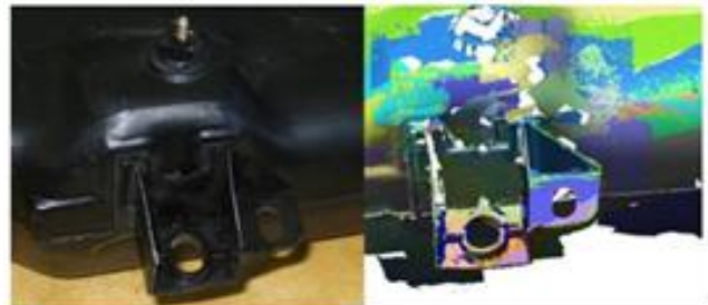
Fig. 2 Petrol tank prepared for 3D scanning.
