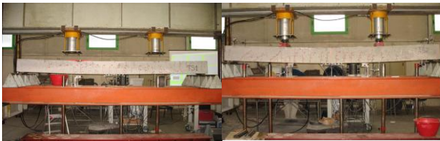
Fig. 6 Beam T1 & T2 - Concrete crushing failure, full cracked section (~90 kN)
