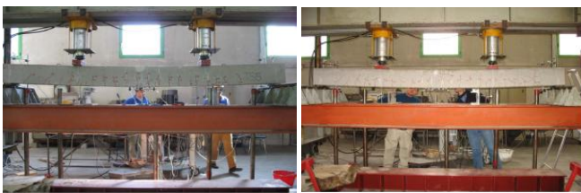
Fig. 7 Beam T3 (~102 kN) & T4 (~55 kN) - Concrete crushing failure, full cracked section
