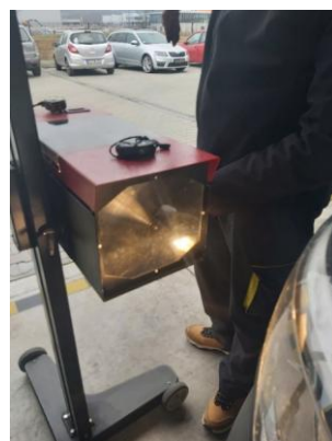
Fig. 4 Display of the mutual positioning and alignment of the central lines of the optical box and the headlight
