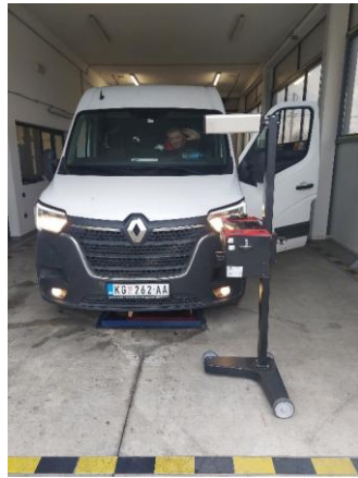
Fig. 2 Example of the work environment, horizontal surface, and the relative positioning of the vehicle and the "Regloscope"
