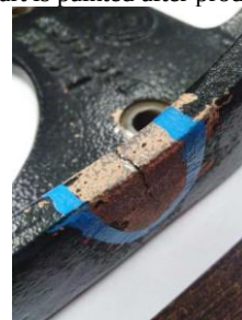
Figure 2 Crack on the specimen
