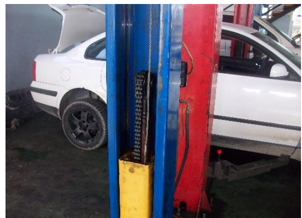
Fig.3. Foto of the of the Main Post, Chain drive and Carriage on the Hydraulic Lift
