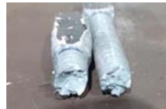
Figure 14 Fractured surface of tensile specimen
