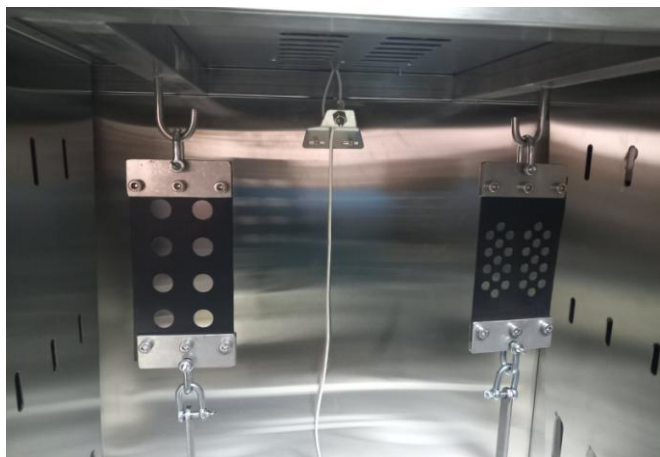
Fig. 4 Installation of the samples in the chamber
