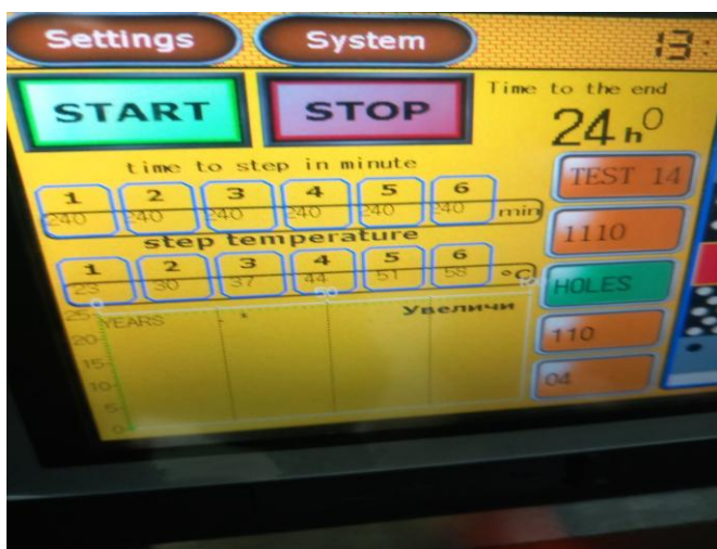
Fig. 5 Parameters of the creep testing
