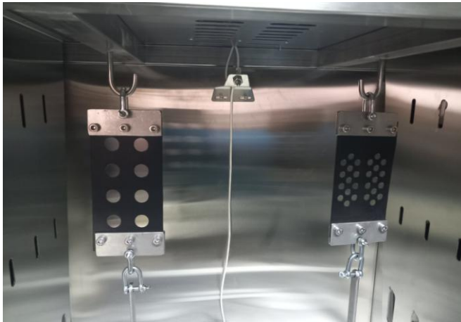
Fig. 4 Installment of the samples in the chamber
