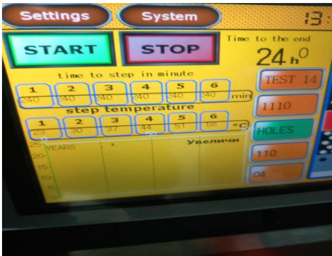
Fig. 5 Parameters of the creep testing
