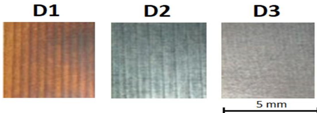
Fig. 1. Optical microscope image of TiO 2 /Ti structure after irradiation by the laser doses D1, D2, and D3 at laser intensity 52.8 MW/cm 2 .
