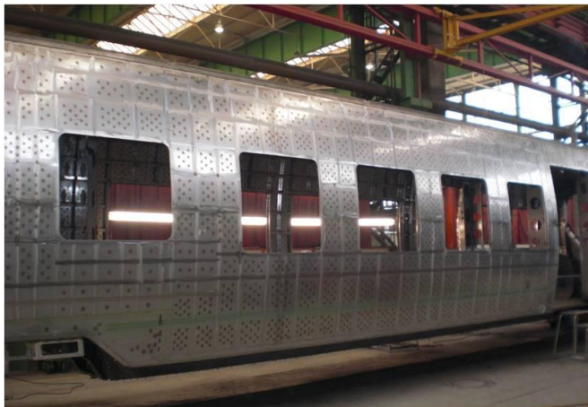
Fig. 1 Railway carriage after thermal straightening, ©ALSTOM Transport Deutschland GmbH, Salzgitter[1].
