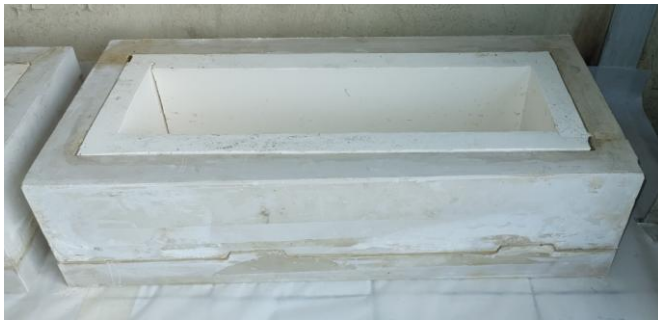
Fig. 2. Formwork mould for the preparation of composite specimens.
