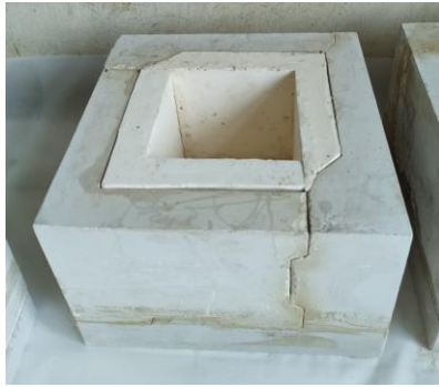
Fig. 1. Formwork mould for the preparation of composite specimens.
