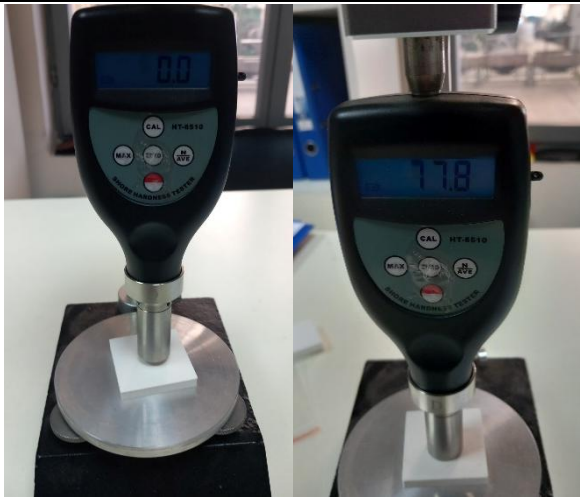
Fig. 2 Measurement of the test specimen.
