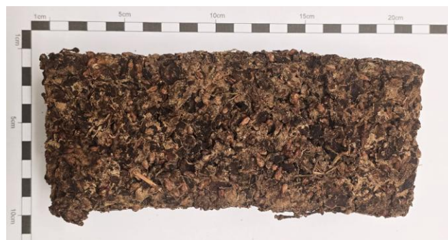
Fig. 1. Dried briquette produced from pressed fermented grape pomace.
