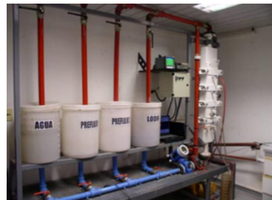
Fig. 3 Device for laboratory testing of mud cake removal quality [22]
