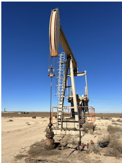
Fig. 3 Mechanical walking beam balanced with counterweight
