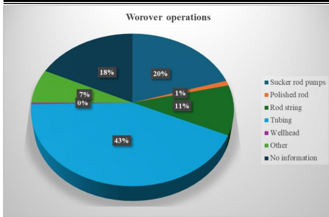
Fig. 8 Workover operations during the period from 2011 to 2022 in relation to the part of the production system in failure
