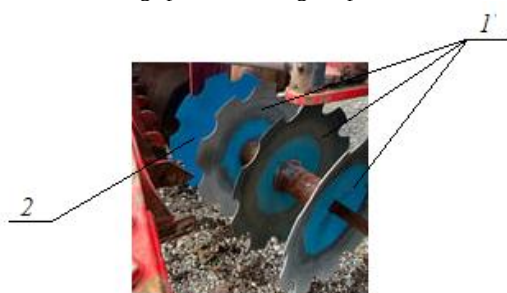
Figure 2. Installed testing discs on the harrow before field testing: 1) three coted discs; 2) uncoted discs.
