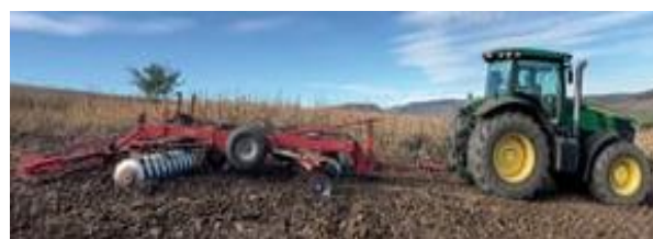
Figure 3. Tractor and 4-metre OTMA disc harrow during stubble field work
