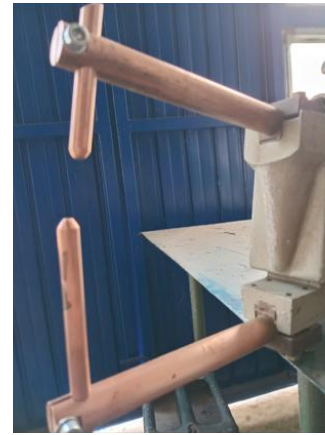
Fig.2 Electrodes for pressure and resistance spot welding
