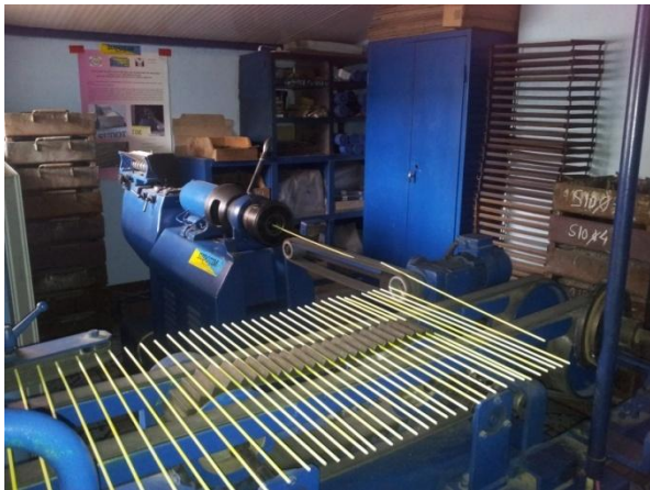
Fig.3 . Manufacturing line rods WRAPPED for brazing .
