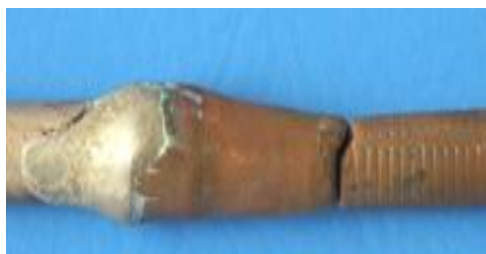
Fig. 6. Tensile test specimen for steel pipe-to-copper pipe joint.
