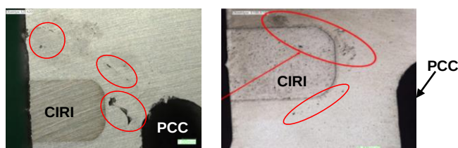
Fig. 4. Macrostructures of an improper insert-piston joint: (a) shrinkage cavities between the insert (CIRI) and the piston cooling channel (PCC); (b) porosity around the insert (property of Federal-Mogul Gorzyce sp. z o.o.).
