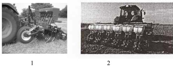
**Fig.4. Machines from „Strip-till“ technique:** 1-strip till subsoiler; 2- twin rows planting machine, [3,4]
