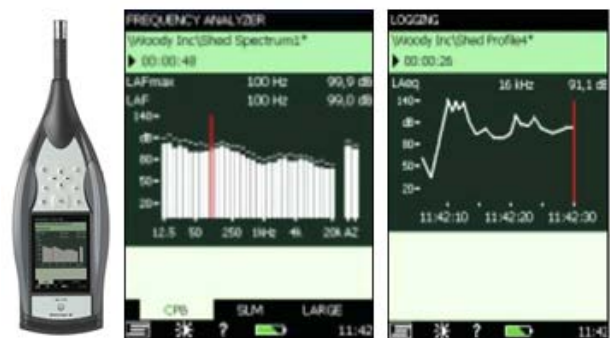
Fig. 3: Hand- held Analyzer Type 2250, module for frequency analysis and time module
